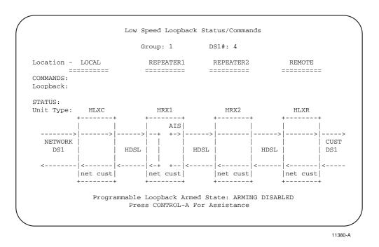
Figure 541-9b. HRX1 Network Loopback Screen (Two HRXs)
